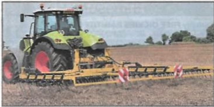
JEFF CLAYDON uses this 7.5m straw harrow operating at up to 25kph to help control weeds and slugs
