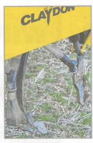
THE PATENTED twin-tine system uses a leading tine for digging and forming a shallow trench of loosened soil, followed, in-line, by a second tine fitted with lateral wings which is used to plant the seed in the trenches formed by the leading tine
