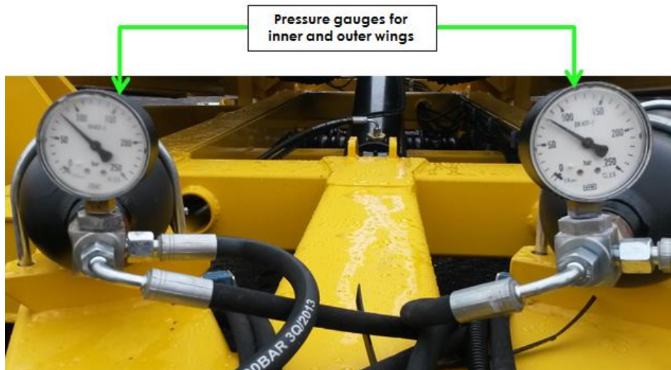
Figure 5: Both pressure gauges should read 80 Bar once unfolded
