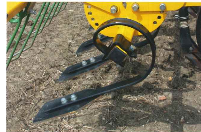
The paddles 'ski' along the surface firming the soil immediately above the seed to ensure soil contact. A light set of spring tines provide the finishing touch.
