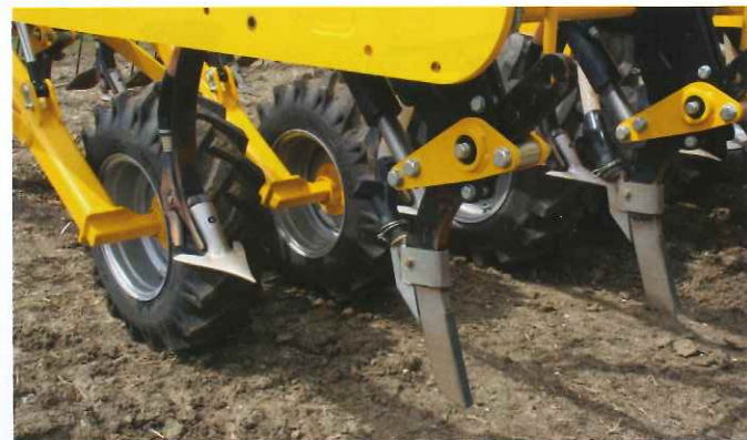
Ground is opened up by the leading rigid tine before the surface soil is moved again to allow the seed to be sown in a band behind it. Note the wheels which support the tool frame and not the seed hopper.
