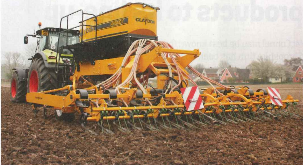
New Claydon 6m and 8m trailed drills have 5,500-litre (4t) hoppers that can be split 60:40 for seed and fertiliser.
