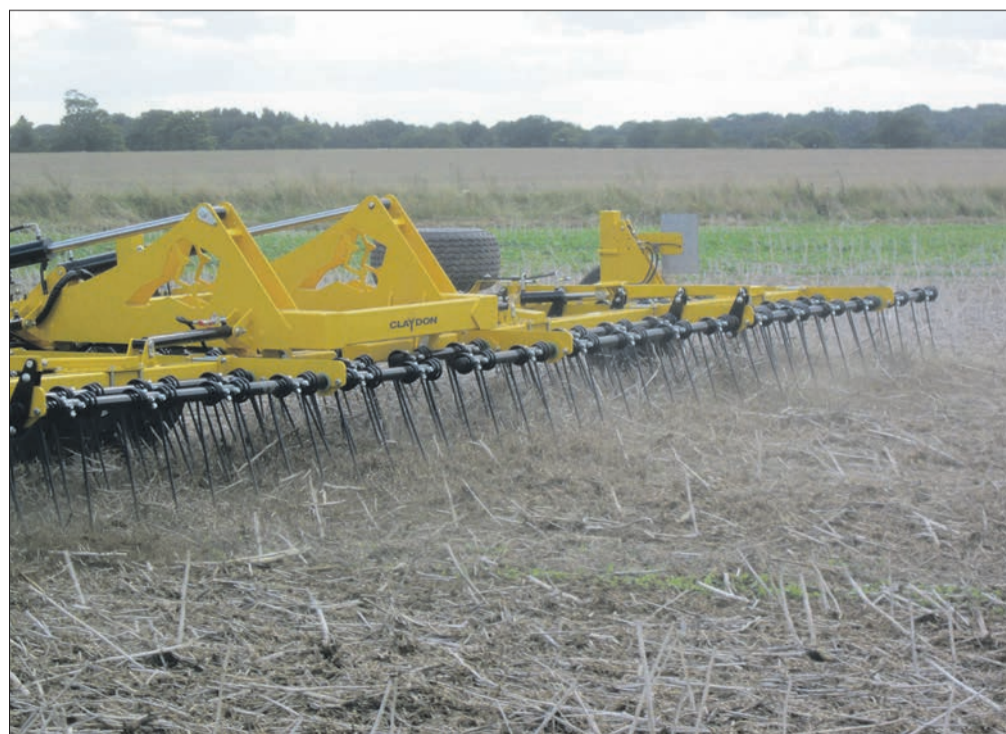
The 15m Claydon straw harrow has twice the output of the Edgeleys' previous 7.5m machine.
