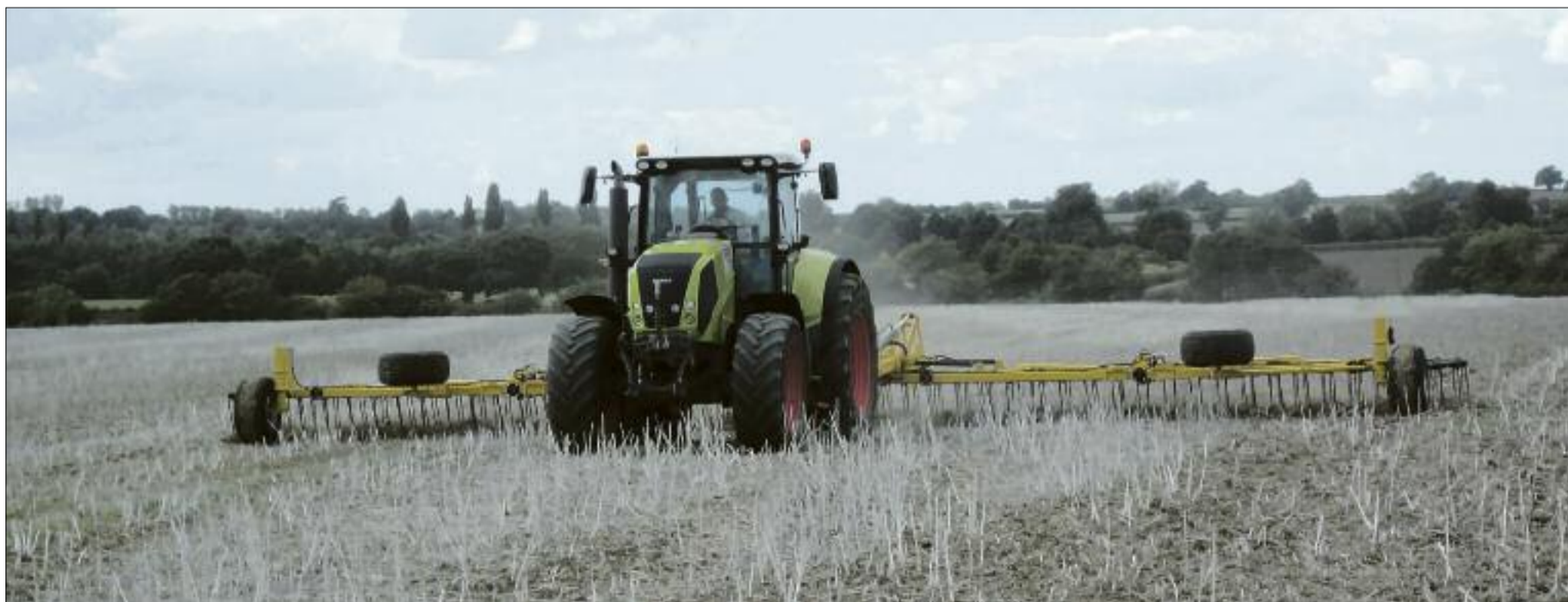
When compared to what the Edgeleys would have spent on glyphosate and slug pellets, it quickly justified the cost of buying the larger 15-metre Claydon straw harrow in autumn last year.
