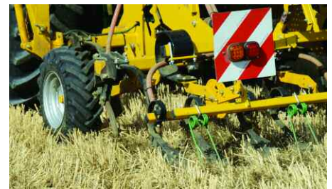
The combination of the tines and rear levelling boards leave a level finish.
