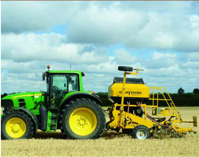
The John Deere 7530 tractor has power in reserve and achieves a daily output of up to 45ha drilling OSR with the 3m Claydon Hybrid.
