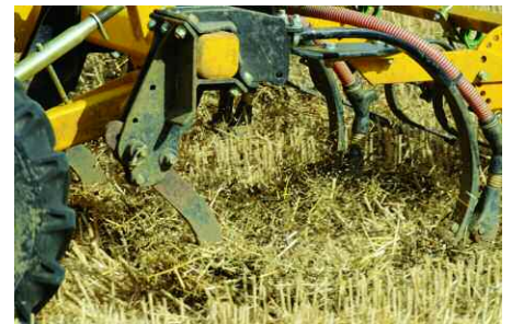
The leading tines are operated at 12.5cm depth for the majority of situations, while seeding tines are adjusted as necessary.
