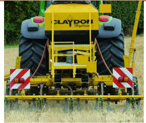
Oilseed rape being drilled into Corn Brash soil at 660mm row spacing with a 3 inch spoon, to reduce soil disturbance.
