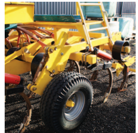
The twin-tine kit comprises two low-disturbance tines which follow the main breaker tine in sequence, and can be retro-fitted.
