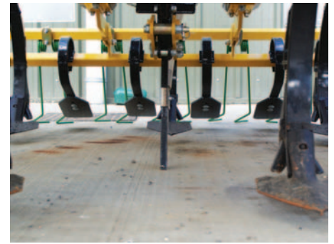
The batterboards are offset so that they skim the soil back over the seed rows, leaving a level, even surface across the width.
