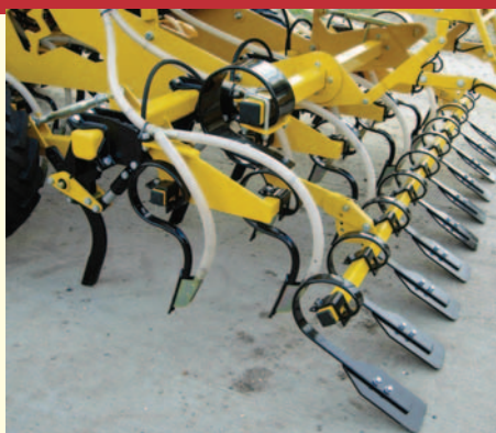
The twin-tine kit comprises two low-disturbance tines which follow the main breaker tine in sequence, and can be retro-fitted.
