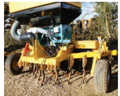
One of the original V-Drills, with tines at 300mm spacings attached to one fixed frame.
