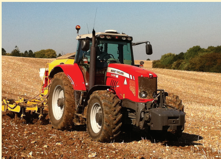
The estate's Massey Ferguson 6499 puts 245hp in front of the drill, which is just enough to manage the slopes, while it now has a 1.5t weight in front to balance the heavy drill.
