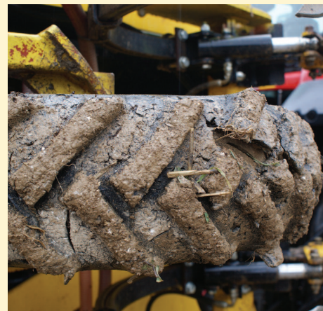
The tyres are foam-filled, while a set of leading tines will only cover 600ha.
