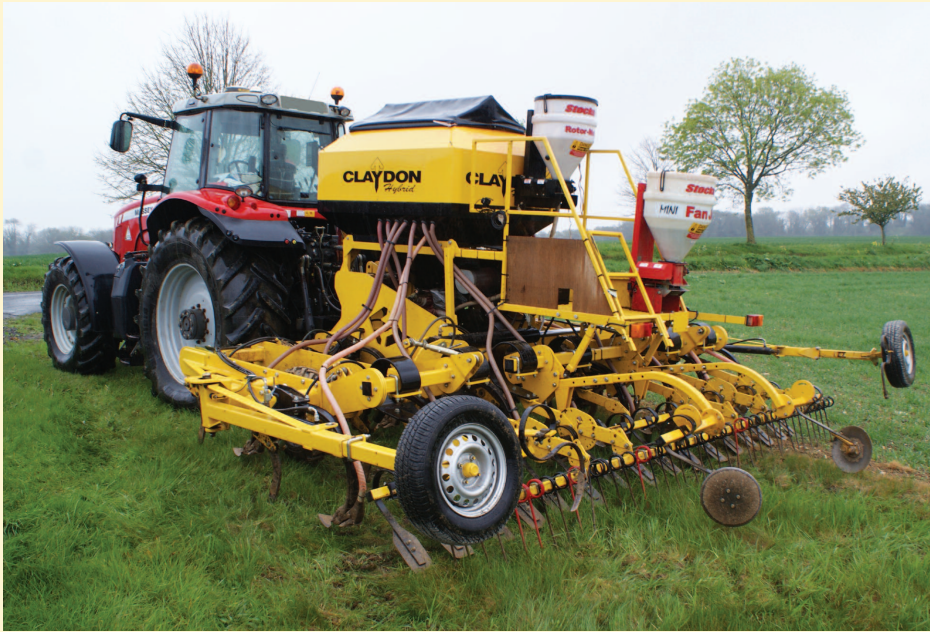
The Claydon Hybrid drill has been fitted with a micro-fert kit for applying Primary-P to the OSR and a slug pellet applicator.
