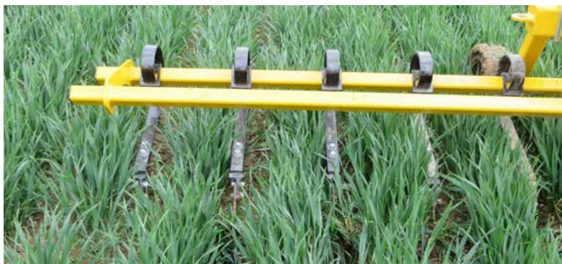
Claydon TerraBlade inter-row hoe. Image courtesy of Claydon.
