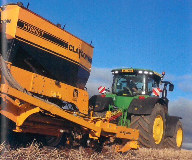
The 6m working width of the Claydon drill quickly folds into 3m-wide transport mode
