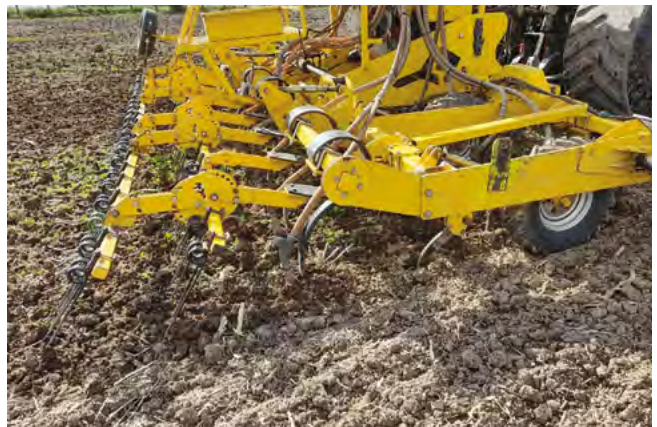
When delivered, the Claydon Hybrid drill was fitted with levelling boards and a rear harrow, but now runs just two rows of harrows.
