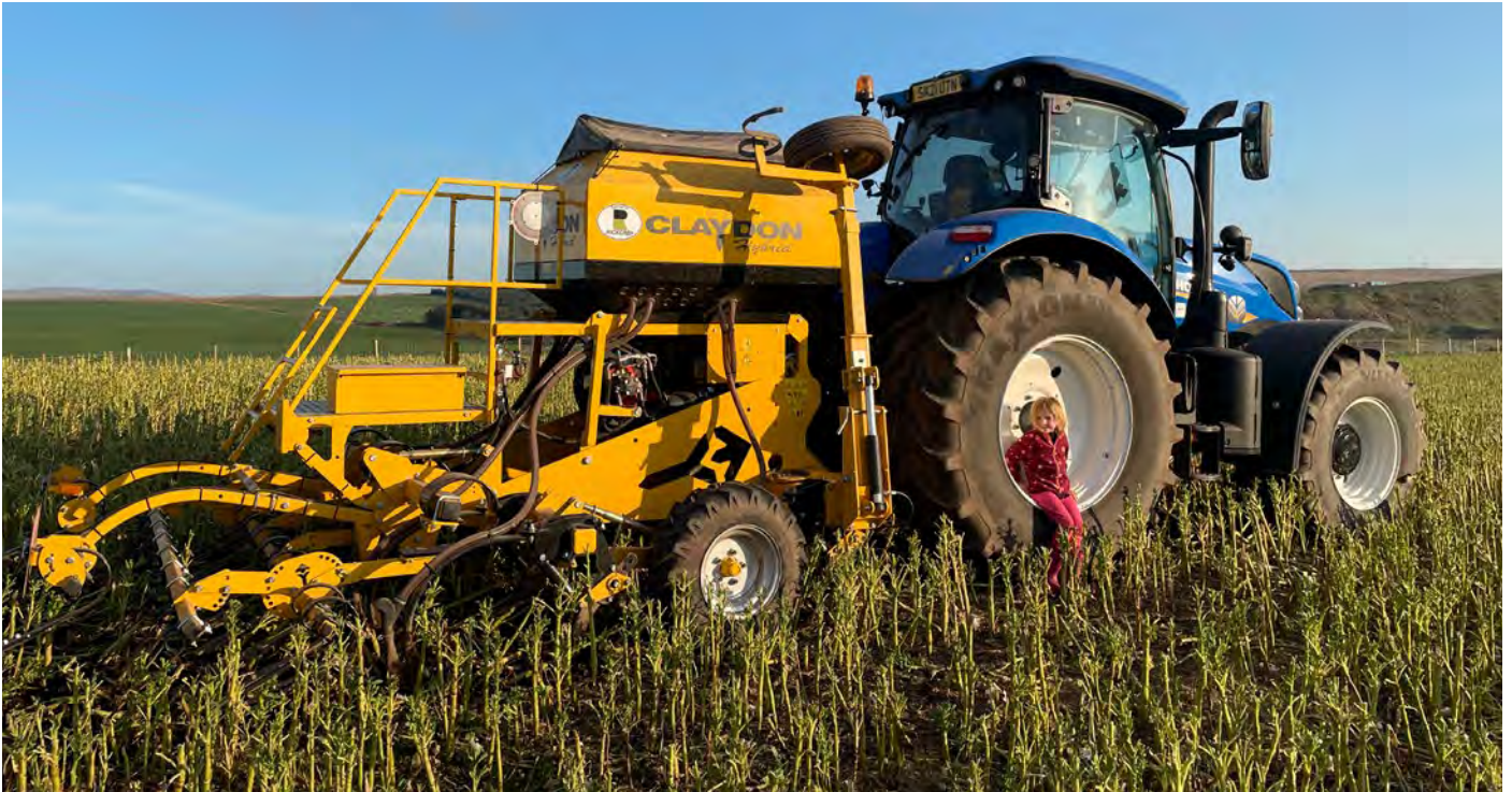
Drilling winter wheat directly into a cover crop using the 3m Claydon Hybrid. In addition to traditional cover crops Penicuik Estate also grows 20 to 25 acres of environmental green manure crops which are sown in May, mulched in September, then drilled with winter wheat. In this situation, the Hybrid's standard leading tines can be replaced with front discs, which are easy to fit and reduce the power requirement even further.
