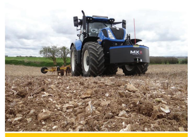
The New Holland T7.260 could pull the Claydon drill much faster but Peter chooses a forward speed of 9 – 10 km/h to minimise wear on the tungsten tine tips and ensure accurate depth control.
