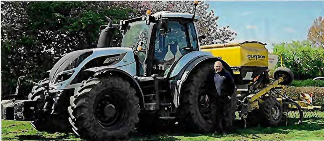
The combination of a relatively light tractor and drill worked well, even on tightly compacted clay soil.
