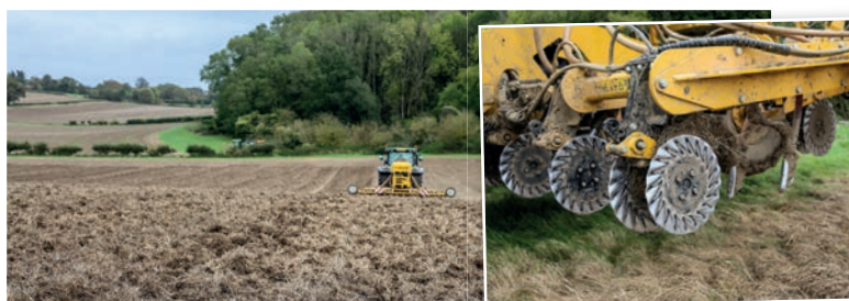
Discs are rarely used due to many fields having a high flint content, but for drilling into grass stubbles they replace the standard leading tines. Operator David Eales, who farms with his father David and Uncle Stephen, said the discs cut through the sward creating a slot for the following tine seeding coulters and avoid peeling back the top layer which can leave open channels.
