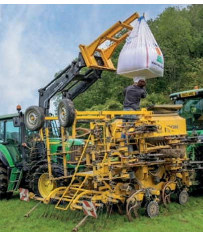
David says the drill is well designed. Filling is easy, the hopper is accessible and calibration through the in-cab display is simple and accurate. It is also quick and easy to swap the working components for different crops and conditions.
