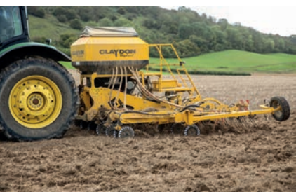
The Claydon 4.8m drill easily achieves work rates of 25–30ha per day. The mounted format is preferred to the previous trailed drill as it improves timeliness and allows greater accuracy when working into field corners.
