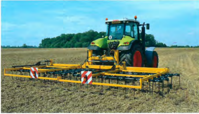
The Claydon Straw Harrow produces a fine 10mm-30mm tilth which encourages weeds and volunteers to germinate
