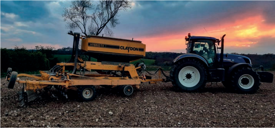
The Strands' Claydon Hybrid T4 is fitted with opening discs, batter boards and twin rear harrows.
