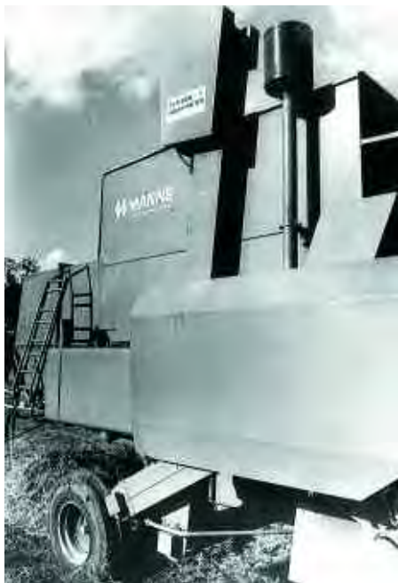
The Yield-o-Meter was Claydon’s founding innovation — which was also claimed to be the first-ever on combine grain monitoring device.
