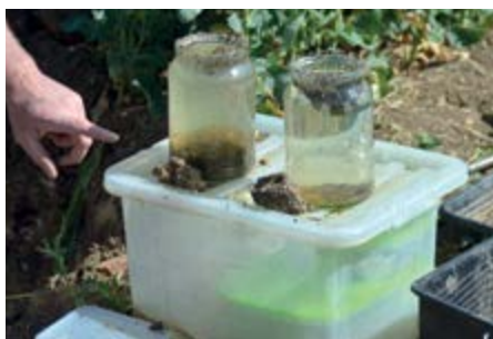
The Slake Test in action. The wire mesh in the jar on the right contains a sample of soil from a field on the Claydon farm which held together firmly even over a prolonged period, so little fell to the bottom and the water remained clear. In contrast, the sample of silt soil in the other jar quickly fell apart and dropped to the bottom, clouding the water.
