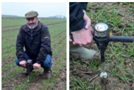
Jeff Claydon tests for compaction in a field of winter wheat during February. Even when inserted to full depth, around 60cm, the penetrometer reading remained in the green, indicating a lack of compaction.
