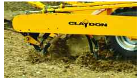
New lower disturbance options are available in place of the leading tine, including disc openers designed for direct drilling into cover crops.
