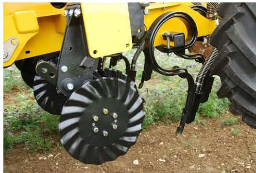
Claydon offer this LD Twin Tine and double Spiradisk set-up as an alternative to the standard leading tine and 7" A share.
