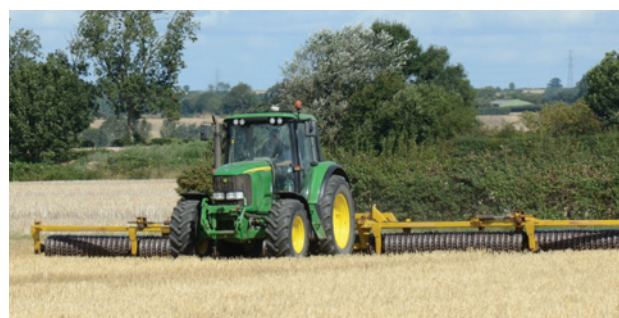
Rolling is an essential part of the Claydon System. Here, Mike Davies carries out the first of two passes with a 12m set of rolls with clod breakers, weighing 10 tonnes which are very good at consolidating and breaking any oversized clods. The crop is ideally rolled within two hours of drilling to establish a really firm contact between seed and soil and to primarily conserve soil moisture.
