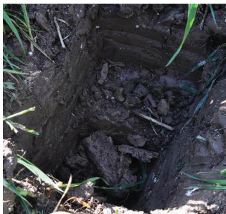
Digging down into the heavy clay soils reveals the sort of stuff that could be used to make bricks.
