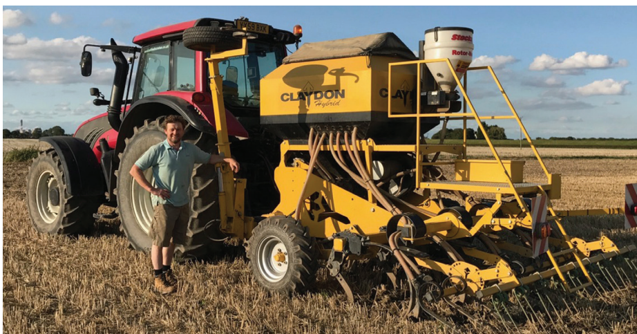
Mark Duckitt and his 3m Claydon Hybrid Drill which he has been using since 2014
