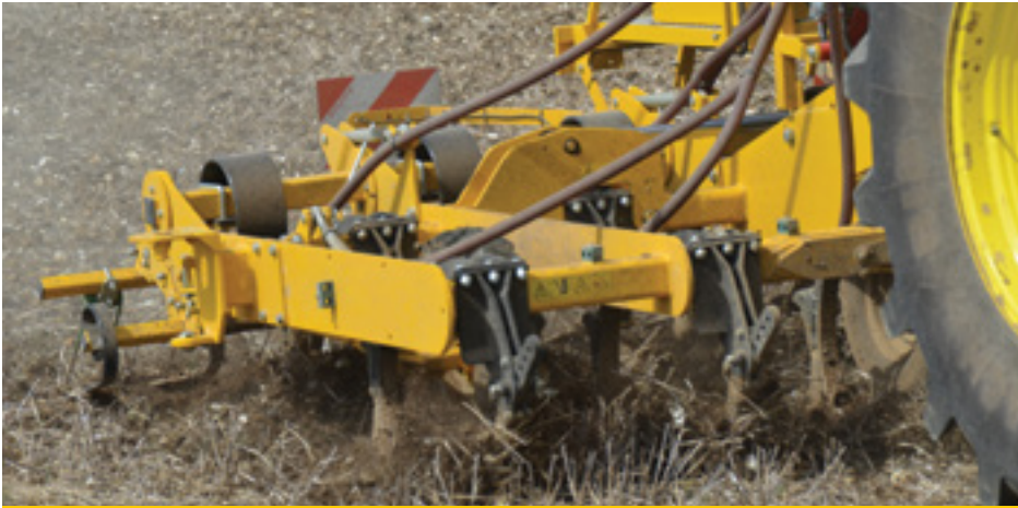
Claydon leading tines lift and aerate the soil - but only in the seeding zone - creating a moist tilth and the perfect growing environment
