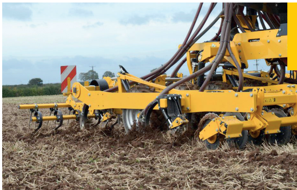
The new 4.8m Claydon Hybrid trailed drill features front shouldered discs, which allow it to work effectively directly into cover crops.
