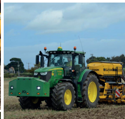
This 215hp John Deere 6125R is used to pull the 4.8m Claydon Hybrid drill at 10-11 km/h, which had been found to give the best results and optimum soil cover behind the rear levelling boards and harrows.
