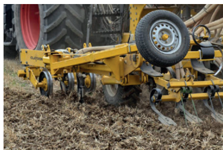
Shouldered discs help to support the weight of the machine and keep it level, while the following tines bust out compaction and let air into the soil before seed is drilled.
