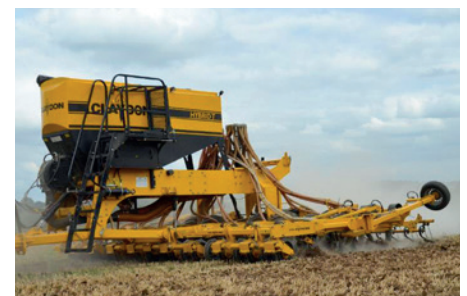
Shouldered discs help to support the weight of the machine and keep it level, while the following tines bust out compaction and let air into the soil before seed is drilled.
