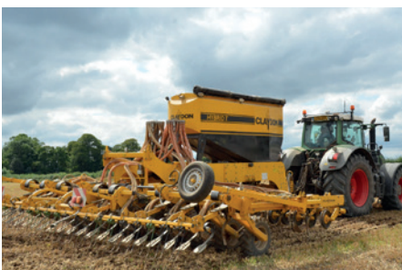
Shouldered discs help to support the weight of the machine and keep it level, while the following tines bust out compaction and let air into the soil before seed is drilled.
