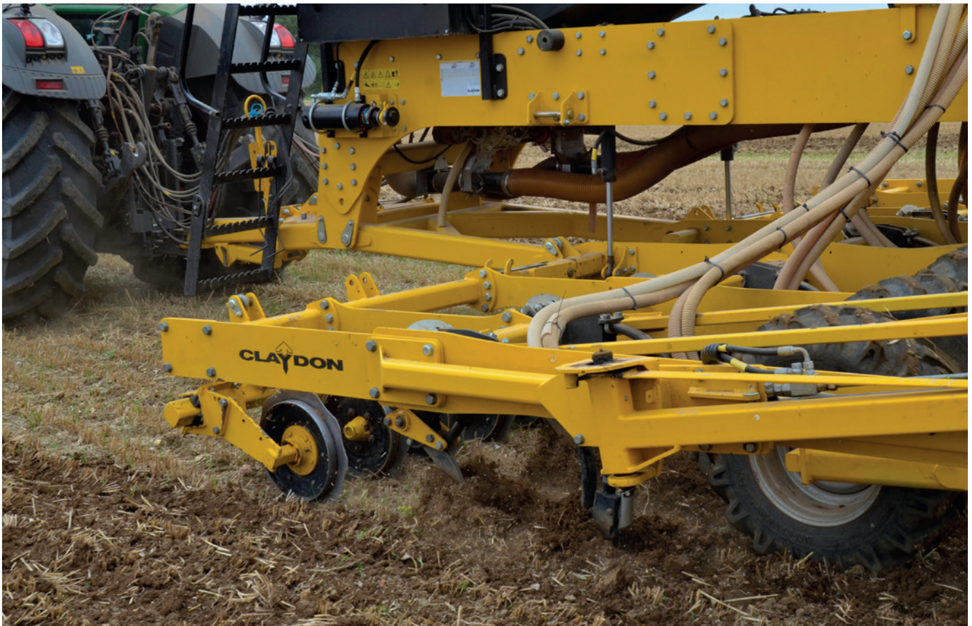
Shouldered discs help to support the weight of the machine and keep it level, while the following tines bust out compaction and let air into the soil before seed is drilled.
