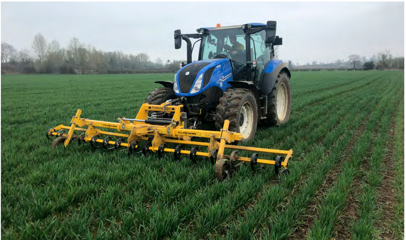
Adrian Taylor's 4.8m Claydon TerraBlade operating in a crop of wheat. The 4.8m version was chosen as it matches the width of the drill and fits in with the farm's 24m tramlines.
