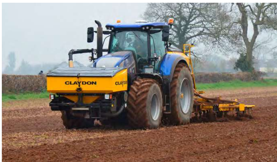
The 1750-litre front tank doubles the seed capacity when drilling in the autumn and carries DAP fertiliser when establishing spring-drilled crops.
